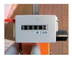
The Nedo Super measuring wheel meets the highest standards in terms of precision, quality and reliability. Thanks to tight manufacturing tolerances and a high-quality counter, its accuracy is  $\pm$  0.02%, which corresponds to a maximum error of  $\pm$  2 cm over a distance of 1000 m.
